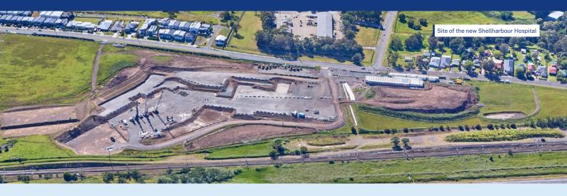
Main works construction for the new Shellharbour Hospital continues to progress, with piling works now completed on site and inground and civil works ongoing. This project is part of the more than \$780 million New Shellharbour Hospital and Integrated Services Project, funded by the NSW and Australian governments.
